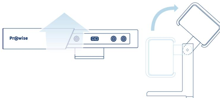
Use the supplied screw to attach the camera to the screen.
