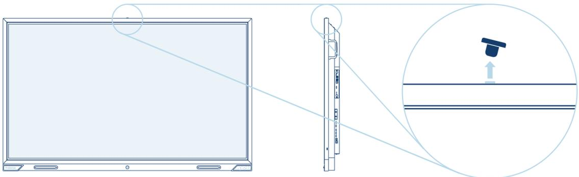
Place the camera (with the Prowise logo facing forward) in the right angle (see image) on top of the Prowise Touchscreen. Make sure that the hole at the base of the camera aligns with the screw hole at the top of the screen.
