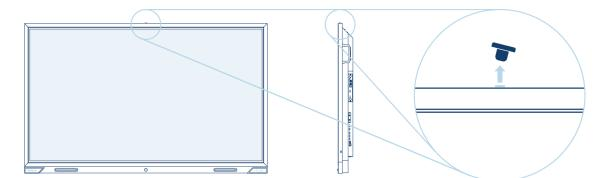
Place the camera (with the Prowise logo facing forward) in the right angle (see image) on top of the Prowise Touchscreen. Make sure that the hole at the base of the camera aligns with the screw hole a the top of the screen.
