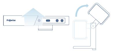
Use the supplied screw to attach the camera to the screen.
