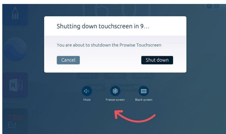
If you press the on/off button for three seconds, a menu appears that can mute, freeze screen or blank screen. As soon as you tap the touchscreen again, you can use it as you normally do.
