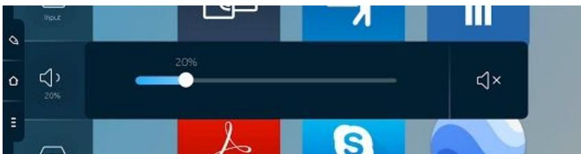
Adjust the volume with this feature of the Prowise Central menu. Drag the dot to the right to increase the volume and to the left to decrease the volume. Click on the mute button to turn off all sound at once. The menu can also be adjusted with the remote control.
