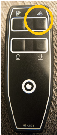
Photograph 9: Tipping unit operating buttons
