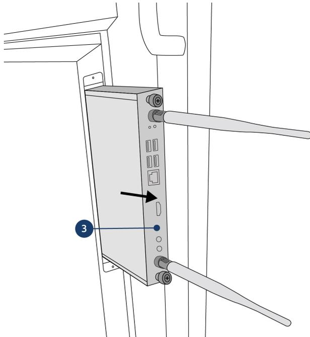
3. Insert the OPS PC module into the slot
