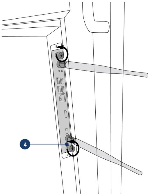
4. Tighten the lock screw of the PC module
