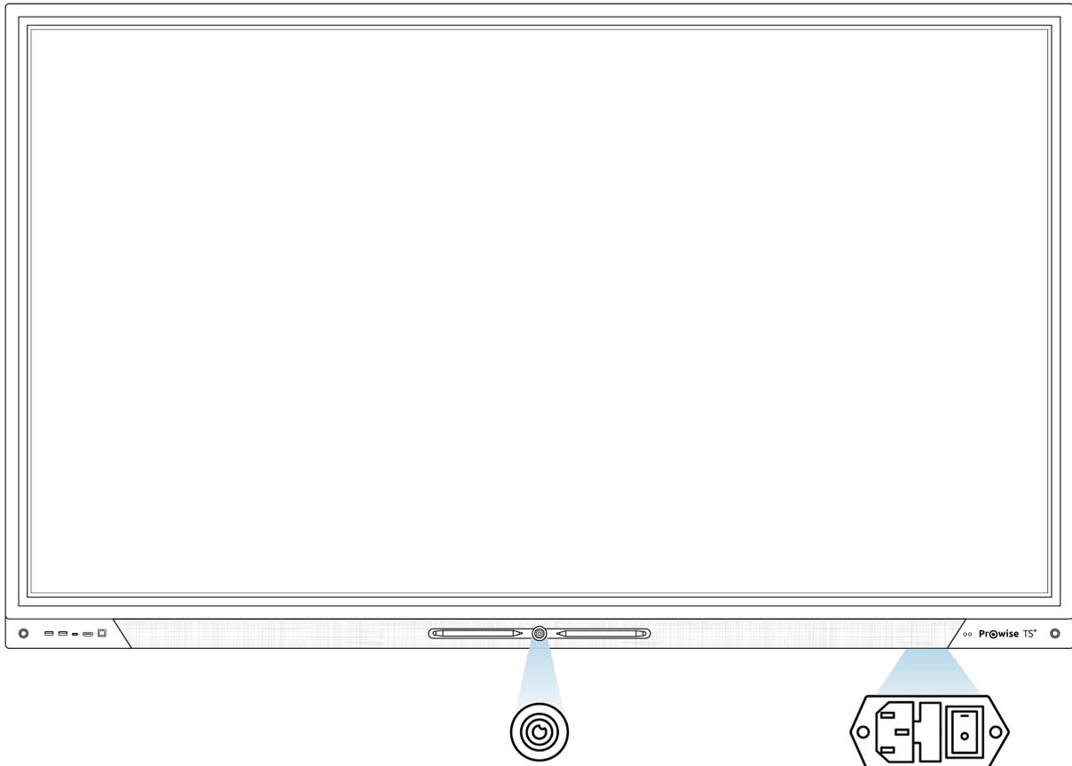
1. Press the control button in the middle of the speaker bar.
