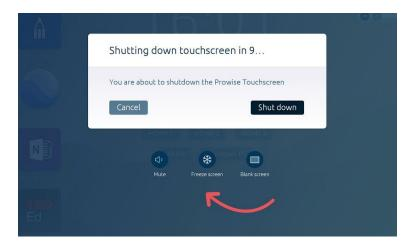
If you press the on/off button for three seconds, a menu appears that can mute, freeze screen or blank screen. As soon as you tap the touchscreen again, you can use it as you normally do.
