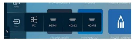
This feature in the Prowise Central menu allows you to change input source. For instance, you can switch from the PC module to the HDMI1 input.
