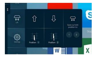
With this menu you can operate the Prowise iPro lift system that is connected to the Prowise touchscreen. The options available depend on the model of the Prowise iPro lift system to which the screen is installed.
