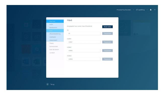
Use this menu to customise the names of input sources. To edit a name, click in the text field, type a new name (up to eight characters) and press 'Apply'. Use the 'Reset all' button to reset the names to the original names of the input sources.
