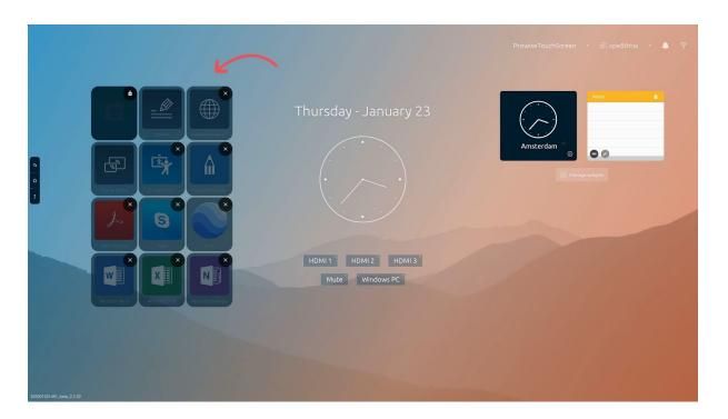
Your installed apps automatically appear in Prowise Central home. Press and hold your finger on an app for two seconds to open the app's settings.
